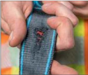
WebAlert™ immediately detects any wear.
