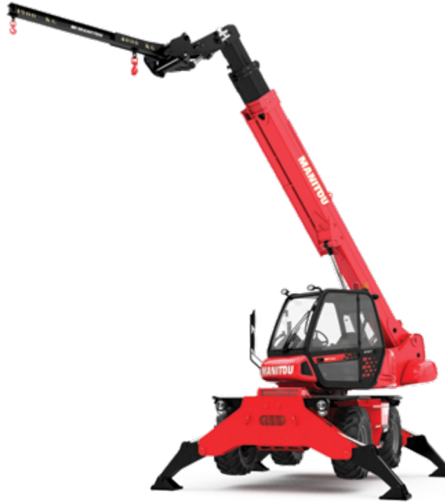
Rotation on lowered stabilisers with 1500 kg jib
