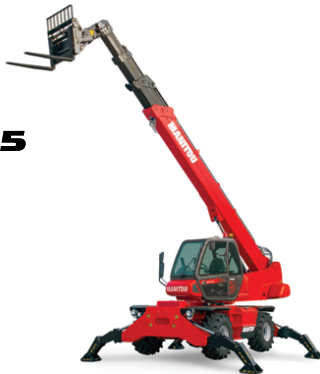
Rotation on lowered stabilisers with forks
